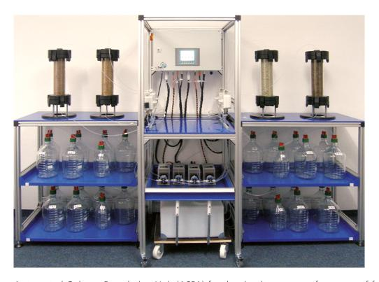
Automated Column Percolation Unit (ASPA) for the simultaneous performance of four separately controlled elution tests; essential components: 4 columns, 4 pumps, 4 hydraulic distributors, eluate bottles, water tank, control module with monitoring function and network connection; completely housed in a custom-made shelving system with full drawers
