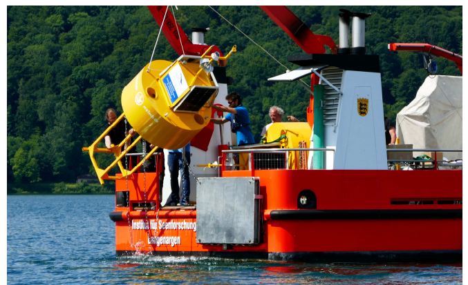
Image. 4: Research vessel "Kormoran" deploying the measuring buoy on site
